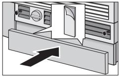
Remove the foil from the adhesive strips.
